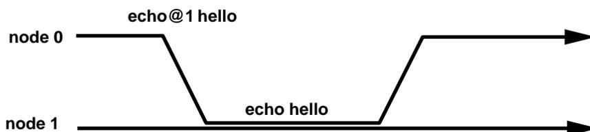
**Figure 21.1** Synchronous Remote Function Call. Node 0 issues the command “echo hello” to node 1, and suspends. When node 1 has executed the command and returned the result to node 0, node 0 continues.
